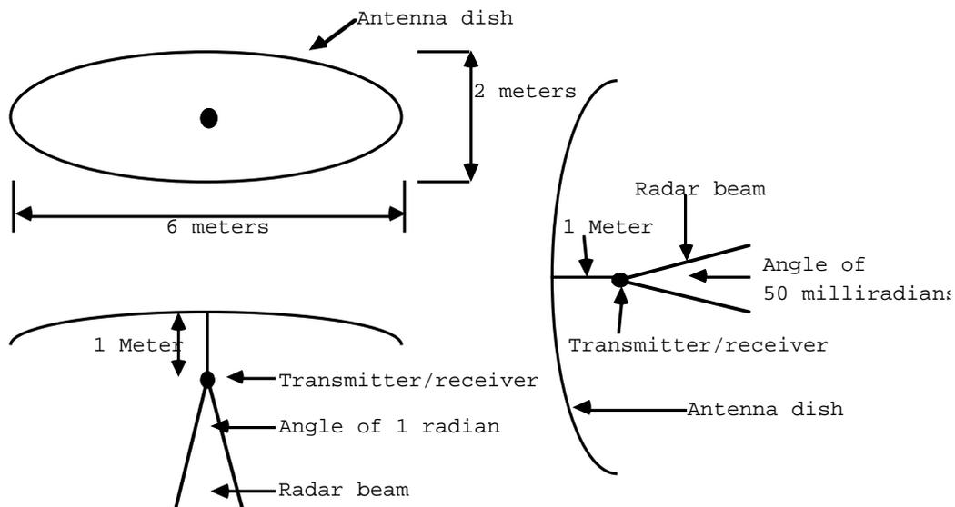
Figure 1. Measurements for the radar system.
