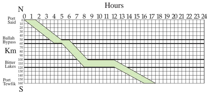
Figure 2: A 10-ship NS convoy moving through the canal.
