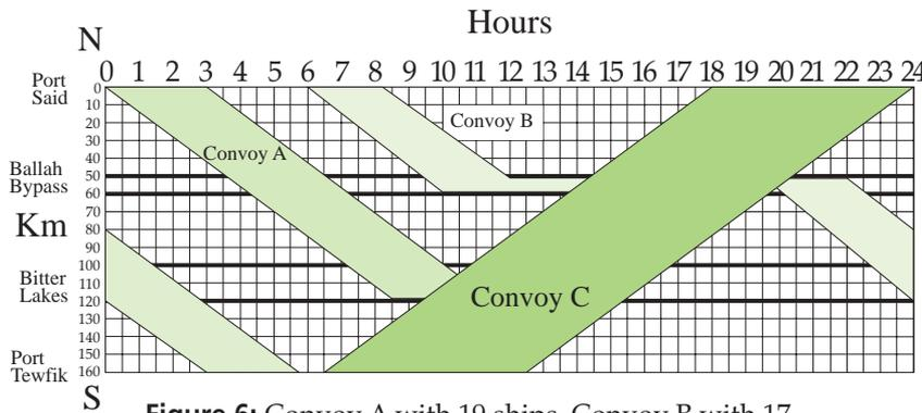
**Figure 6:** Convoy A with 19 ships, Convoy B with 17 ships, Convoy C with 36 ships
